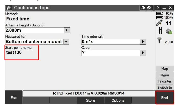
Point id under Start point name will keep increasing (after every 1 second in this case) and once the required number of measurements have been done, click on End.
